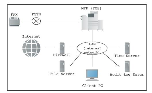
Figure 1 Operational environment of the TOE
