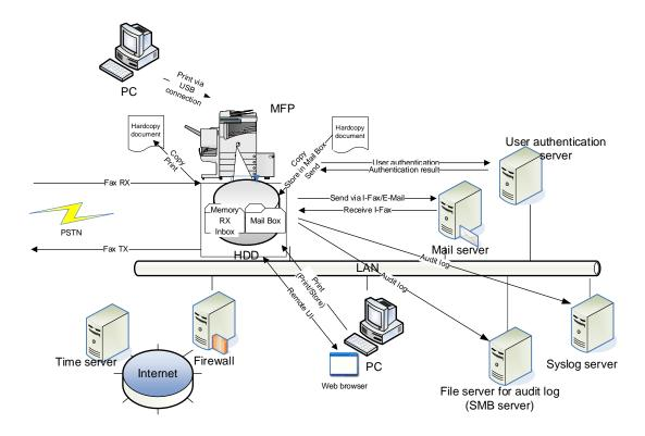
Figure 1 The assumed operational environment of the MFP < Canon imageRUNNER ADVANCE DX C357/C257 Series with Fax>
