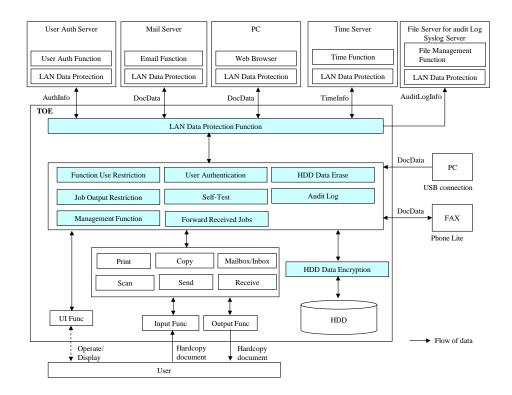
Figure 3 Functional configuration of the TOE
