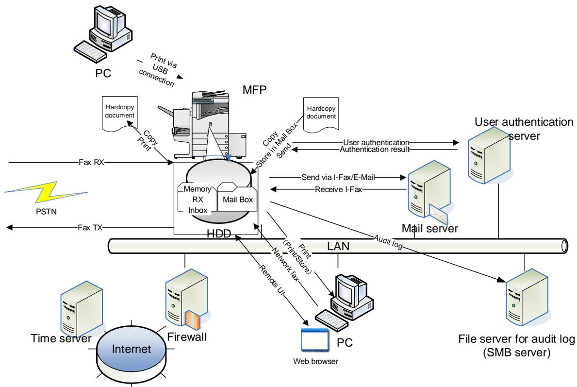
In Figure 1, the MFP is connected by an internal LAN, to all of the other major components, namely the Mail Server, User Authentication Server, File Server for Audit Log (SMB Server)<sup>1</sup>, PC, and Firewall. Furthermore, the internal LAN is protected by Firewall from threats from the Internet. To send (via I-Fax or email) a previously scanned document or when receiving a document by I-Fax for example, the MFP connects to the
