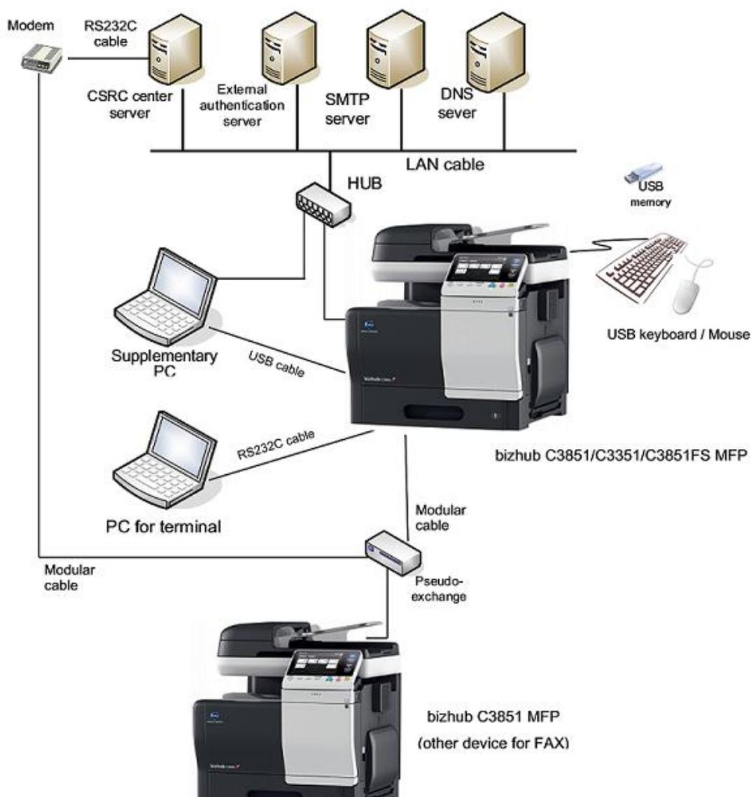
Figure 7-1 Configuration of the Developer Testing
