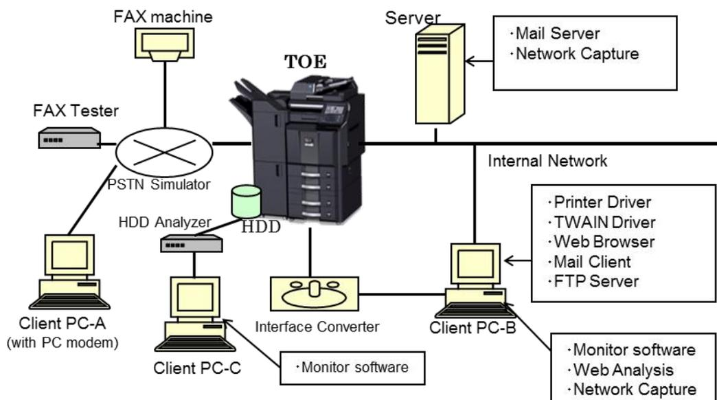
**Figure 7-1 Configuration of the Developer Testing**
