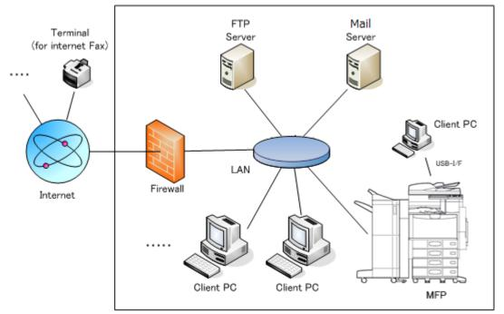
Figure 4-1 Operational Environment of the TOE
