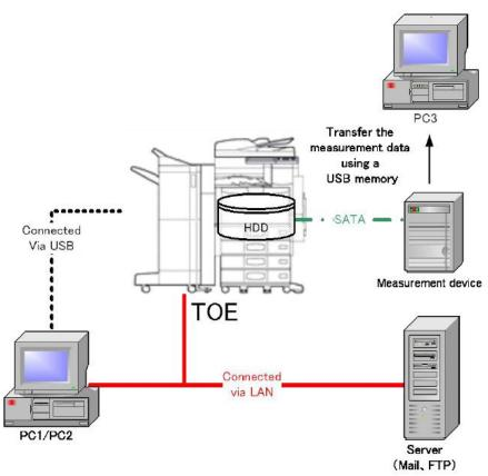
Figure 7-1 Configuration of the Developer Testing
