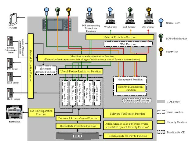
Figure 3 : Logical Scope of the TOE
