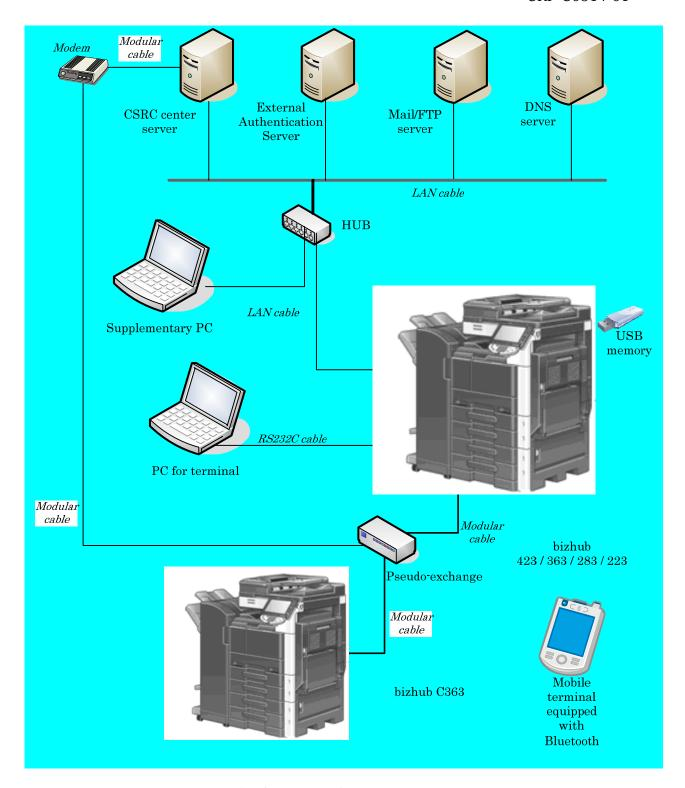
Figure 7-1 Configuration of the Developer Testing
