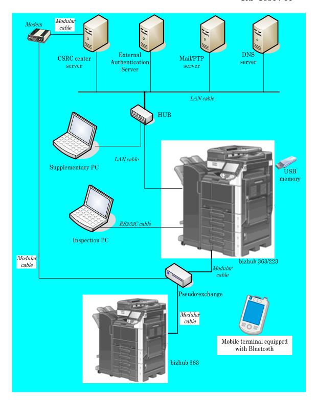
Figure 7-2 Configuration of Penetration Testing
