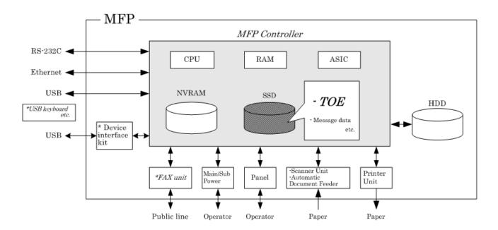
Figure 2 Hardware composition relevant to TOE
