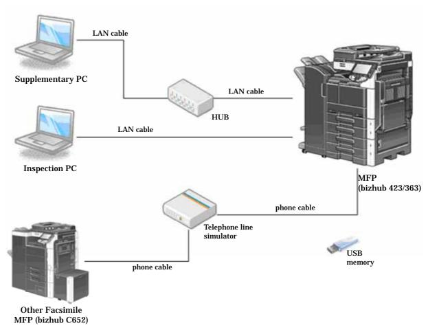
Figure 7-2 Configuration of Penetration Testing
