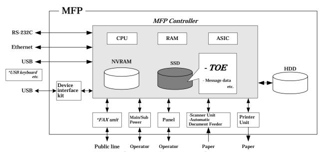
Figure 5-1 Hardware configuration relevant to TOE
