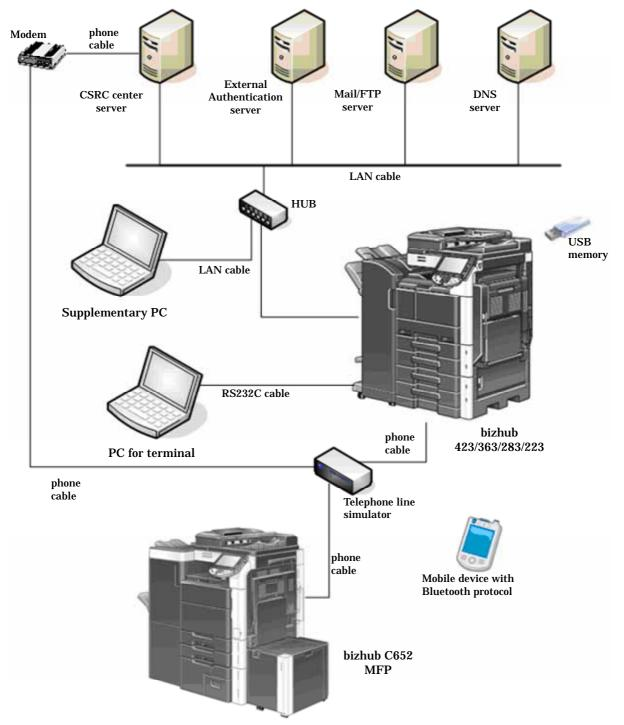
Figure 7-1 Configuration of Developer Testing
