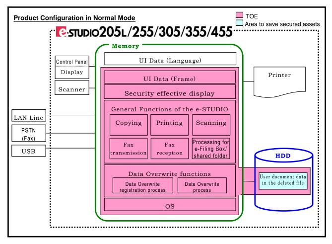
Figure 1-2 Product Configuration in Normal Mode
