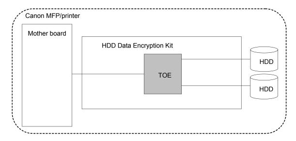
Figure 2-1: TOE usage environment
