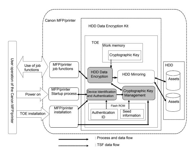
Figure 2-3: TOE logical configuration
