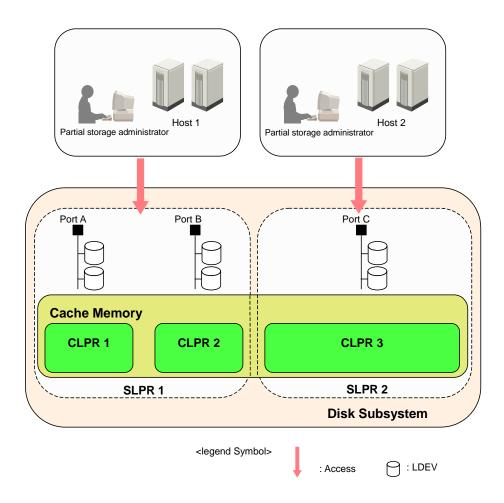
Figure 2.3 Overview of the Virtual Disk Subsystem
