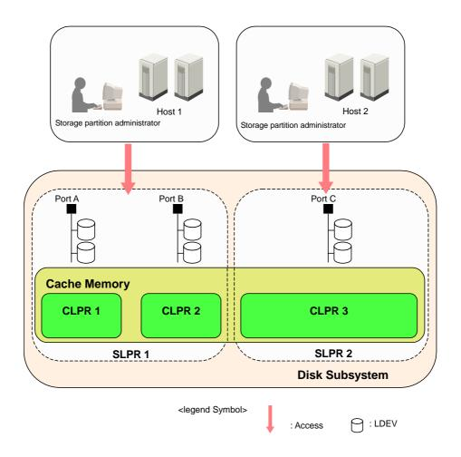
Figure 1.3 Virtual Disk Subsystem
