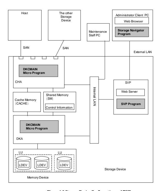
Figure 1.2 Storage Device Configuration and TOE
