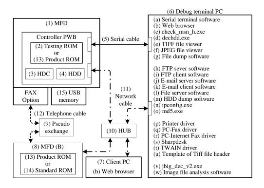
Figure 3-1: Configuration of the Developer Testing
