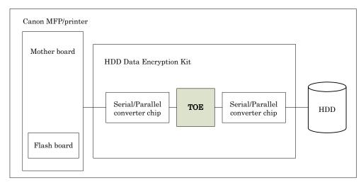
Figure 2-1 : TOE usage environment
