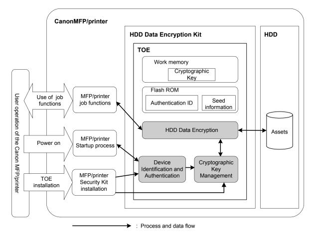
Figure 2-3 : TOE logical configuration
