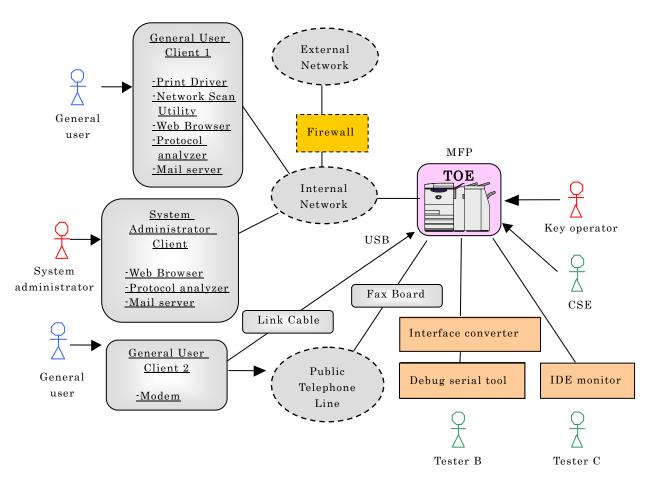
Figure 2-1 Configuration of Developer Testing
