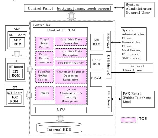
Figure 1-1 TOE Physical Scope and Configuration
