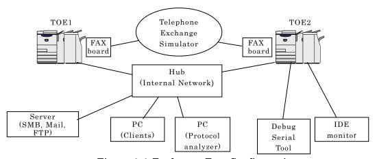
Figure 2-2 Evaluator Test Configuration
