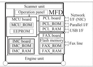
Figure 1: TOE and physical configuration of the MFD
