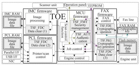
Figure 2: Logical configuration of the TOE
