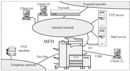
Figure 3: Usage environment of the MFD
