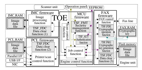
Figure 1-2: Logical configuration of the TOE
