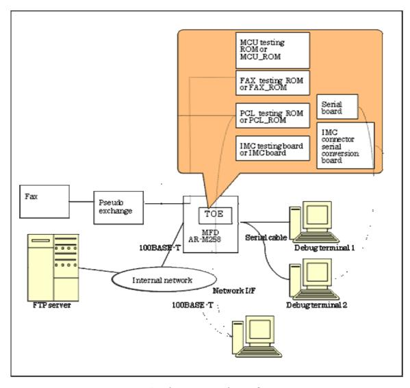
Figure 2-1: Configuration of Developer Testing
