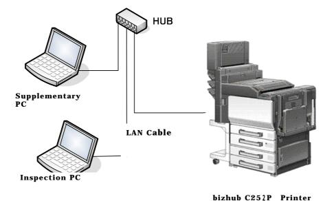
Figure 0-2 Developer test (Intrusion test) configuration
