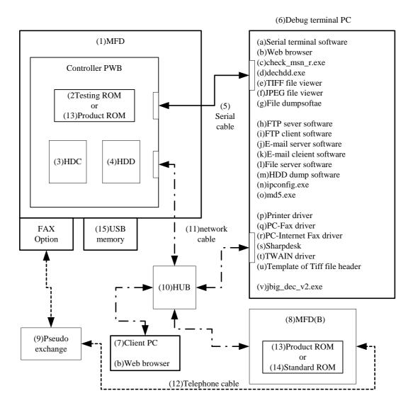
Figure 2-1 Configuration of Developer Testing
