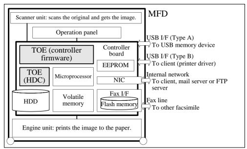
Figure 1-1: The physical configuration of the MFD and the physical scope of the TOE
