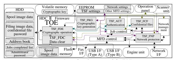
Figure 1-2: Logical configuration of the TOE
