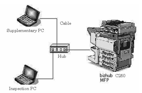
Figure 2-2: Evaluator test (Intrusion test) configuration
