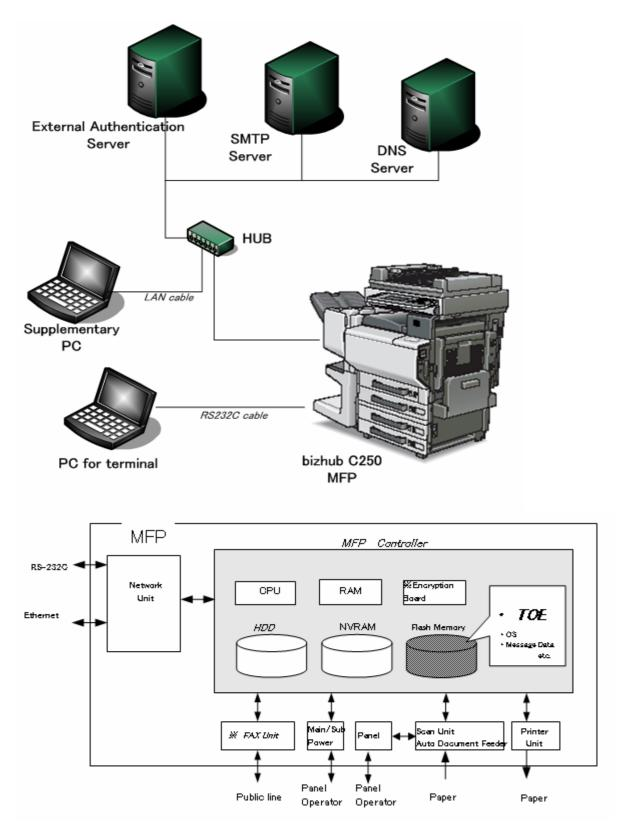
Figure 2-1: Developer test configuration
