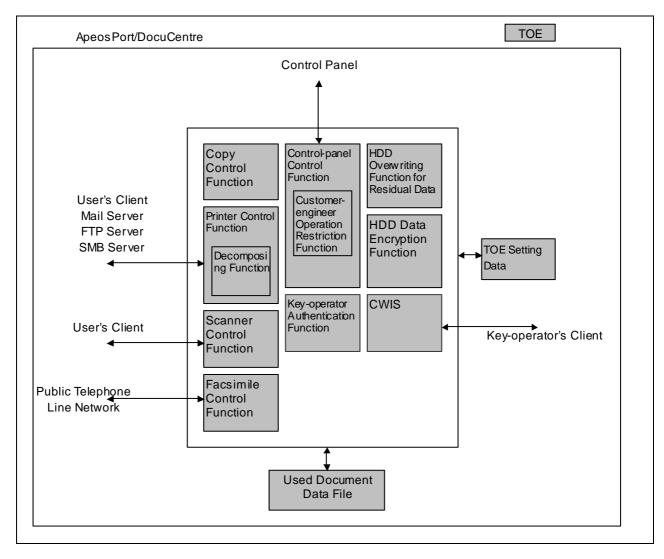
Figure 3: Logical Configuration of TOE
