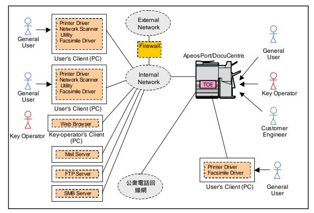
Figure 1: Assumed Usage Environment of TOE
