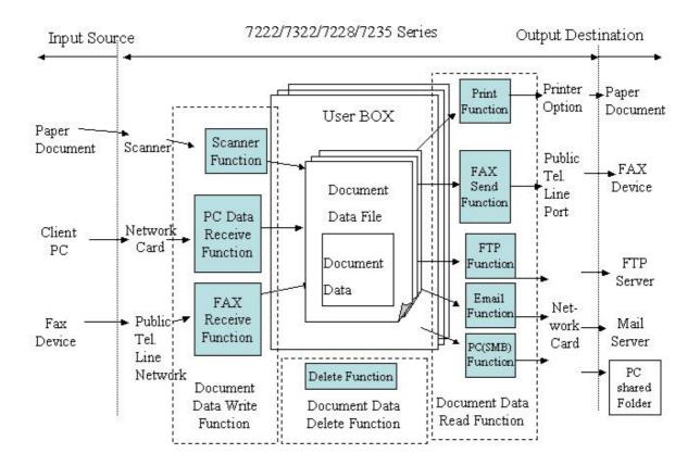
**Figure 2-3. Basic Functions Processing Concepts**
