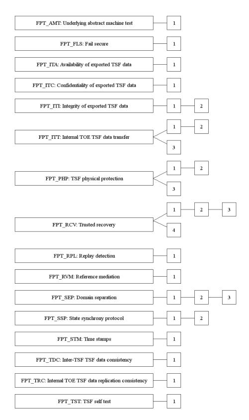
Figure 30 - FPT: Protection of the TSF class decomposition
