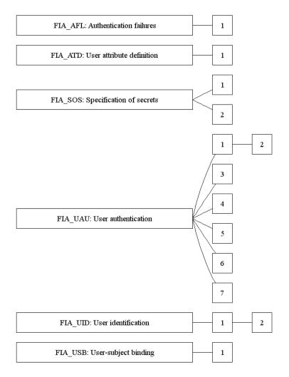
Figure 13 - FIA: Identification and authentication class decomposition
