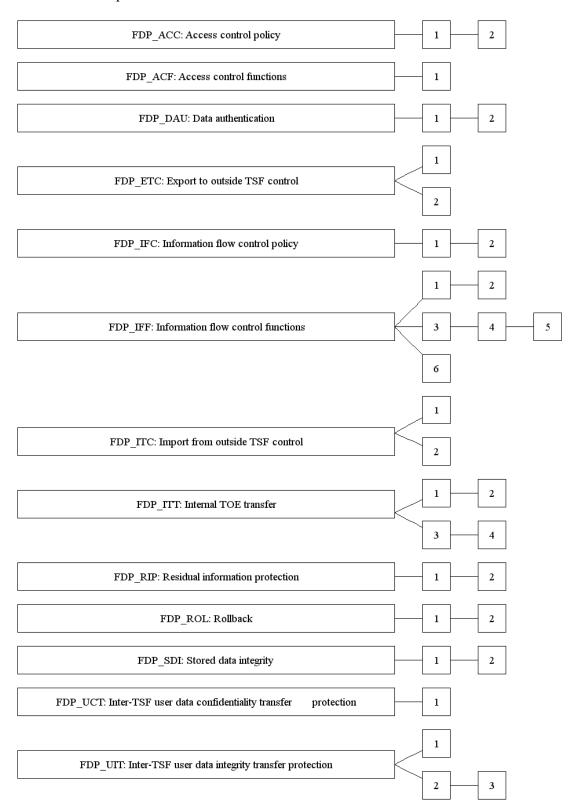
Figure 26 - FDP: User data protection class decomposition
