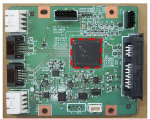
Figure 1 Exterior of Canon MFP Security Chip (FK4-1731A)
