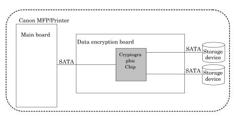
Figure 3 Example operational diagram of Canon MFP Security Chip
