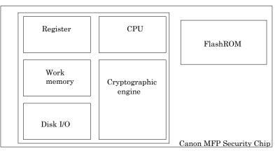
Figure 4 Canon MFP Security Chip component diagram
