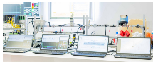
Simulated gas supply plant and HMI screen
