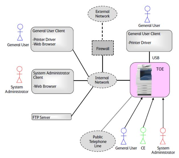
Figure 4-1 Operational Environment of the TOE
