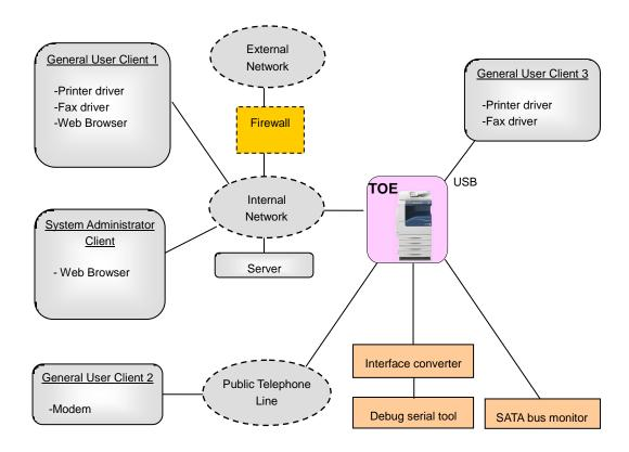
Figure 7-1 Configuration of the Developer Testing
