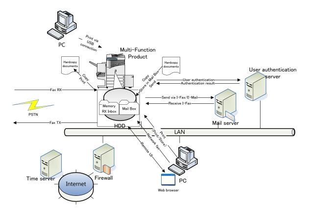
Figure 4-1 Operational Environment of the TOE
