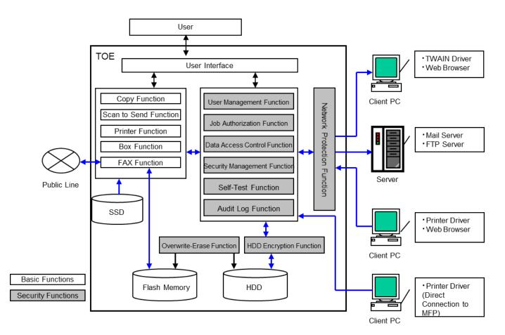
Figure 1.3 Logical Configuration of TOE
