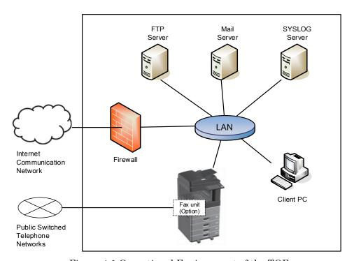
Figure 4-1 Operational Environment of the TOE
