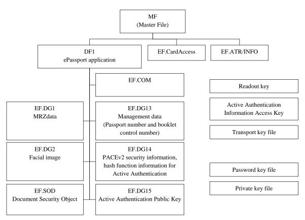
Figure 1-1 File structure of ePassport IC
