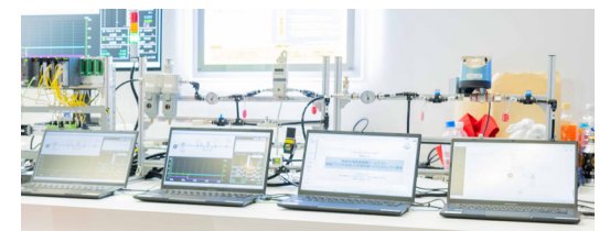
Simulated gas supply plant and HMI screen
