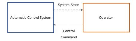
In order to solve issue 1 and 2, it is necessary to not only analyze individual CAs but also to grasp the feature of the system from the Control Structure and to identify hazard scenarios.
