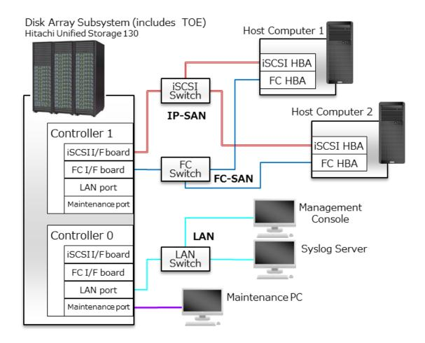
Figure 7-1 Configuration of the Developer Testing
