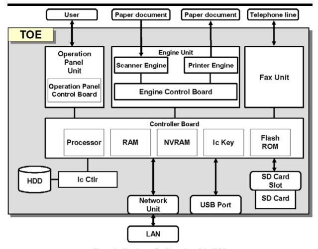
Figure 2: Hardware Configuration of the TOE
