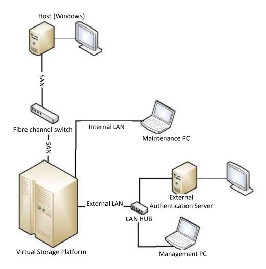
Figure 7-2 Independent Testing Configuration
