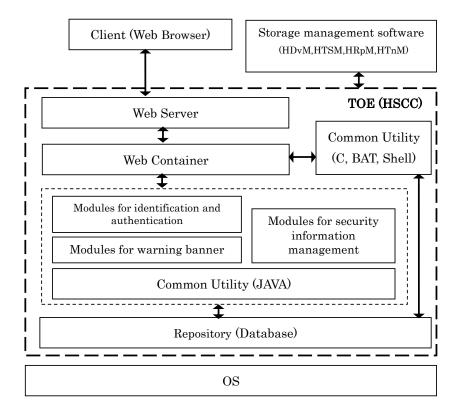
Figure 4: Physical TOE scope (bold dotted line)
