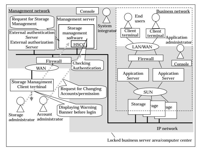
Figure 4-1 Operational Environment and Configuration
