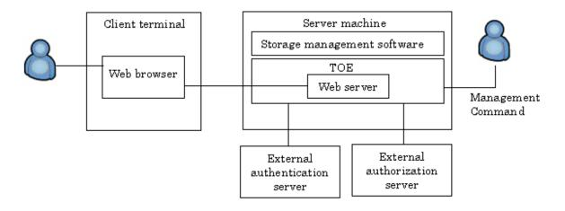
Figure 7-1 Configuration of the Developer Test
