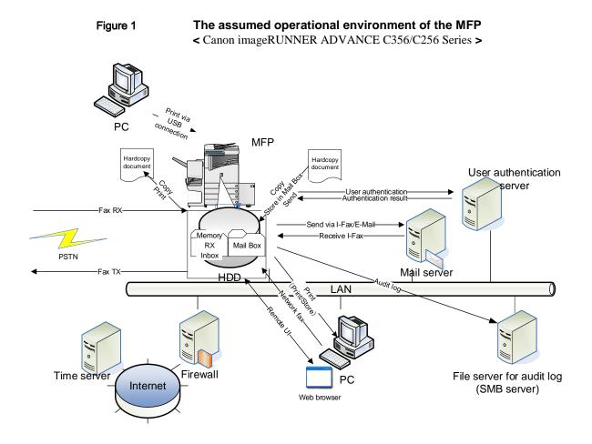
In Figure 1, the MFP is connected by an internal LAN, to all of the other major components, namely the Mail Server, User Authentication Server, File Server for Audit Log (SMB Server)<sup>1</sup>, PC, and Firewall. Furthermore, the internal LAN is protected by Firewall from threats from the Internet. To send (via I-Fax or email) a previously scanned document or when receiving a document by I-Fax for example, the MFP connects to the
