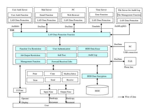
Figure 3 Functional configuration of the TOE
