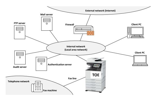
Figure 4-1 Operational Environment of the TOE
