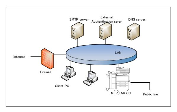
Figure 4-1 Operational environment of the TOE
