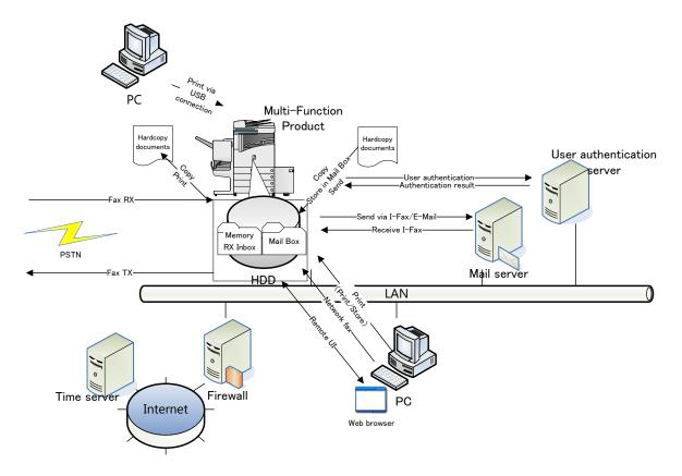
Figure 4-1 Operational Environment of the TOE
