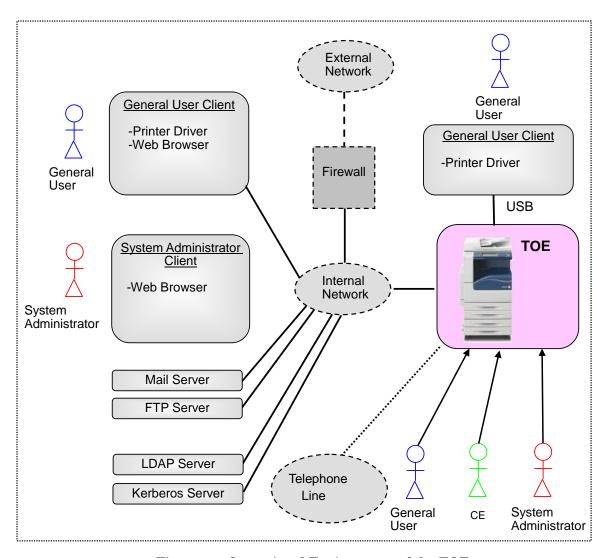
Figure 4-1 Operational Environment of the TOE
