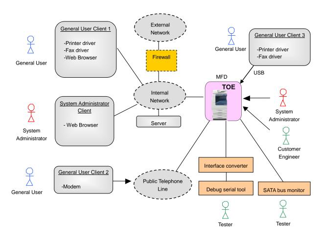
Figure 7-1 Configuration of the Developer Testing
