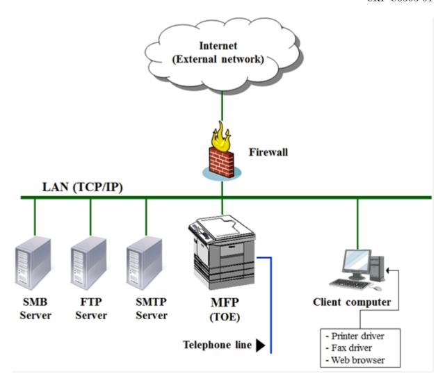
Figure 4-1 Operational Environment of the TOE
