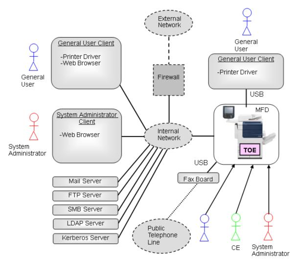
Figure 4-1 Operational Environment of the TOE
