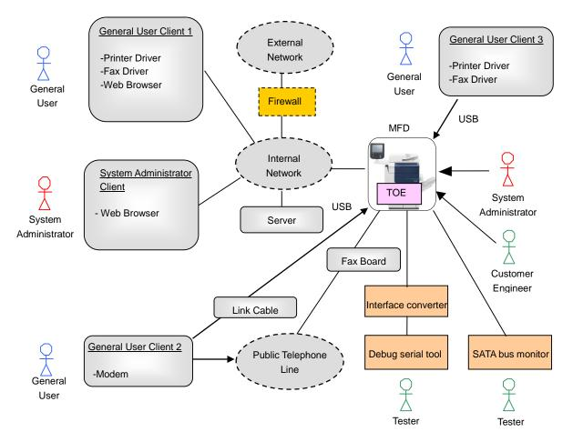
Figure 7-1 Configuration of the Developer Testing
