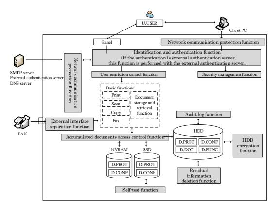
Figure 1-3 Logical scope of the TOE
