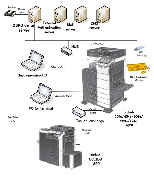
Figure 7-1 Configuration of the Developer Testing
