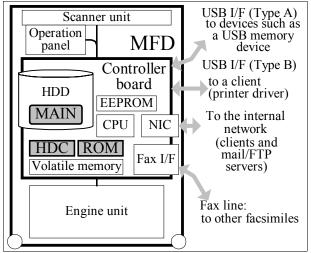
Figure 2: TOE and physical configuration of the MFD K to the HDD in the MFD.
