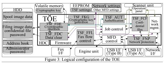
Arrows in the figure indicate data flows. Functions of the TOE usually put data in the volatile memory temporarily to pass the data to each other. However, the figure omits every such detail except security significance.
